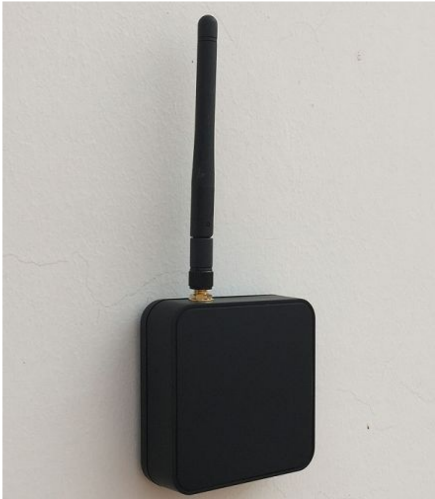
WSN1101L in an enclosure with external Antenna
